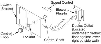
Figure 26 - Attaching Speed Control to Firebox
